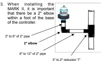
For example: On a 3" vacuum system use a 3" to 2" reduction 'T', connect to the 'T' approximately 6" to 12" of 2" straight pipe, then a 2" elbow, then another 3" to 6" of 2" straight pipe, then install the Mark II on a 2" coupling. FROM ELBOW TO MARK II DO NOT EXCEED 12 INCHES.
